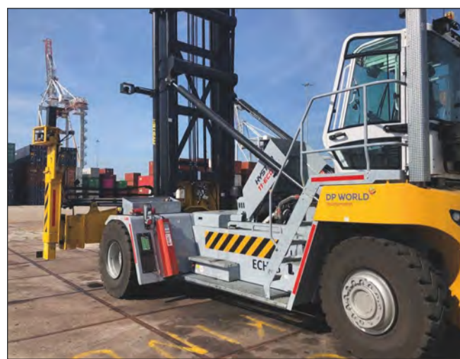
Hyster EC mast truck with Dafo Vehicle's fire suppression system
